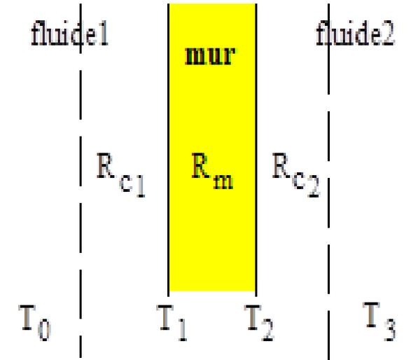
$$R = R_{c1} + R_m + R_{c2} = \frac{1}{h_1 S} + \frac{1}{h_2 S} + \frac{\ell}{\lambda S}$$
